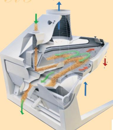
The new generation of machines, with its types TS 90-S, TS 180-S and TS 360-S, are operated with aspiration (no dust escape) and are equipped with the patented flywheel type of drive, ensuring complete balancing of the dynamic forces(= minimum of vibrations).
